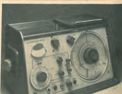
MARCONI TF1313A Universal Bridge L.C.R. 0.1% accuracy. £790 Current new price £995.00
